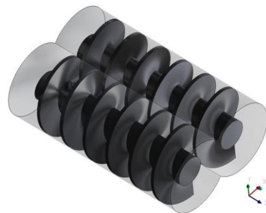
Figure 8: 3D geometry of the twin-screw extruder implemented in ANSYS FLUENT 17.0.
